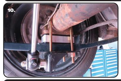
**10.** Tighten the Bushing hardware, torquing it to 75 ftlbs. The Delrin Bushings will not bind, so it isn't necessary to have the car at ride height.
