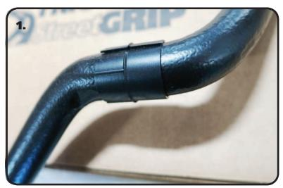
the Sway Bar in the approximate location they will need to be when installing the Sway Bar on the Car.
