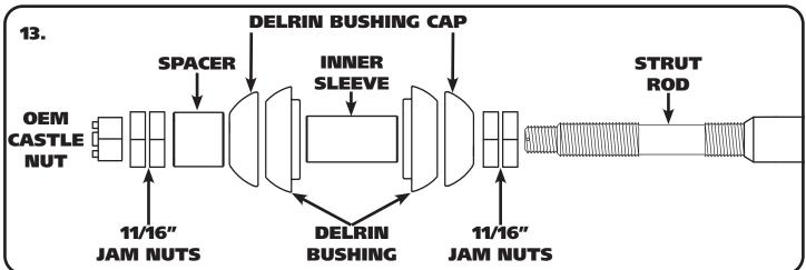
**13**. Install (2) 11/16" Jam Nuts on the INNER THREADS of the strut rod followed by the Delrin Bushing Cap. Insert the strut rod through the Bushing Sleeve until the Ball is nested into the Bushing Cap. Install a second Bushing Cap on the strut rod followed by the Spacer. Next, install the (2) 11/16" Jam Nuts on the OUTER THREADS. Install the OEM castle nut on the end of the strut rod with a cotter pin through it. Position isn't critical, it will be adjusted when the front end is aligned.
