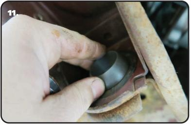
11. Refer to (Image 13) for the Delrin Strut Rod Bushing assembly order. The Delrin Strut Rod Bushing will insert into the frame bushing hole with the rounded side of the bushing outward. A Bushing needs to be installed on both the front and rear side of the frame.
