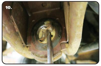
**10.** A Delrin Bushing setup for the strut rod is also included in this kit. The liner that is installed in the frame hole has to be removed. Use a chisel to distort it and remove it. In **(Image 10)** we distorted it from the bottom edge and removed it.
