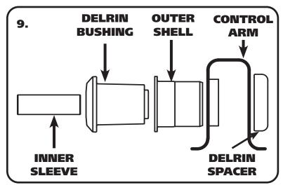
**9.** Install the Outer Shell into the control arm. Next, install the Delrin Bushing into the Outer Shell followed by the Inner Sleeve. With the Delrin Bushing and Inner Sleeve installed, install the Delrin Spacer over the SMALL end of the Delrin Bushing. The ROUNDED surface will be out, away from the control arm.
