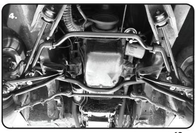
**4.** Slide the Sway Bar into position on the Car. The Sway Bar Arms will be above the Control Arms. With the Sway Bar in position, slide the holes of the Bushing Straps onto the 3/18"-16 studs sticking out of the OEM sway bar mount. With the Sway Bar held in place, install a 3/8"-16 Nylok Nut on each of the (4) studs. Do **NOT** Completely tighten the Hardware. It will be left partially loose until the End Links are installed.
