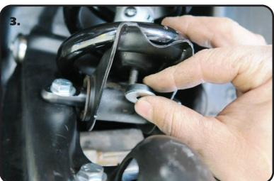
**3.** Using **(Image 5)**, install a Stud Top Bushing Washer and Bushing on the Stud Top of the Shock. Insert the Shock through the OEM opening. Insert the studs into the openings in the lower mount. Using **(Image 2)** as a reference, install a Bushing, Washer and Nut on each stud and tighten.
