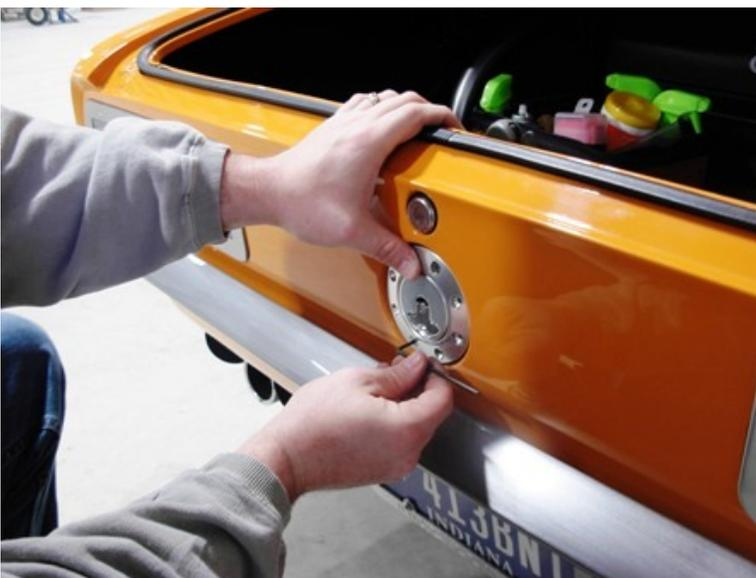
9. Bolt the cap to the filler neck with the 10-32 x 3/4" screws supplied.
