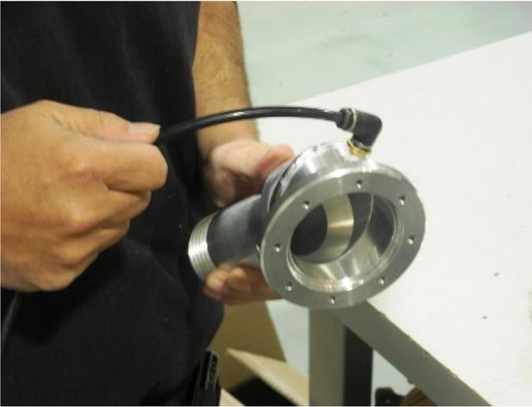
6. Factory gas tanks require a vented gas cap. This gas cap is not vented, but there is an 1/8" NPT hole tapped into the top of the filler neck that can be used to vent the tank. A hose should be used to route the fumes outside the trunk. Most aftermarket tanks are vented though; a 1/8" NPT brass plug is supplied to plug this hole.
