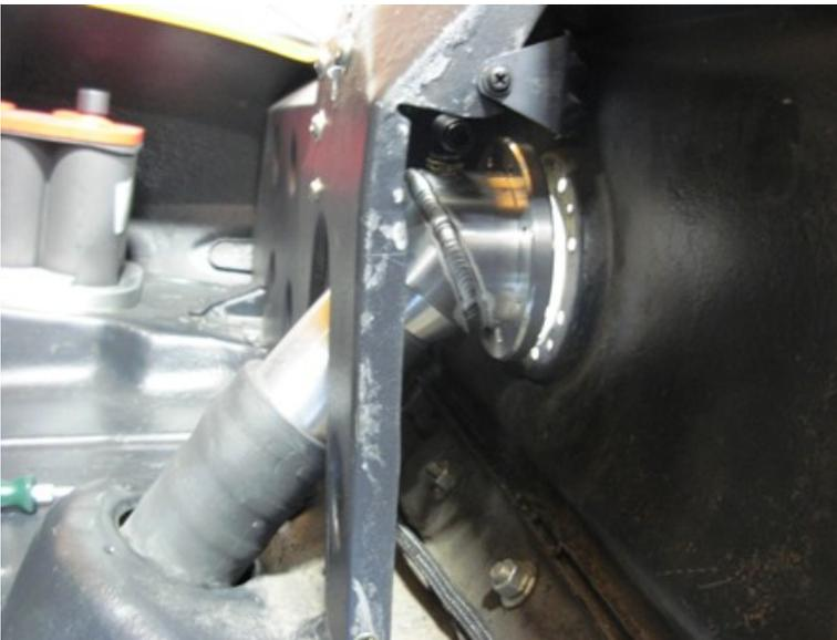
7. Attach the rubber hose to the gas tank with the #36 hose clamp supplied.
