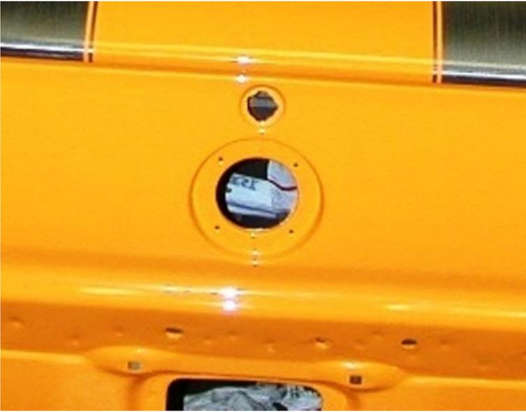
2. The factory filler neck used four screws to attach it to the tail panel. This cap will use 8 screws to sandwich the cap and filler neck to the panel.
