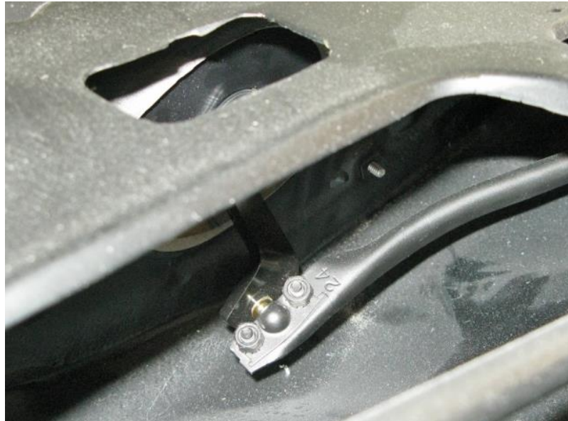
Figure 3 - Attach Pitman Arm to Wiper Linkage
