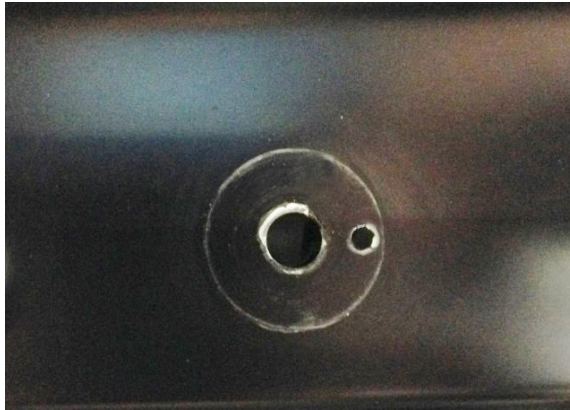
Figure 5 - Drill Anti-Rotation Hole
