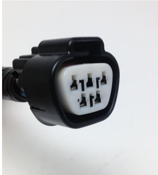
Figure 9 - Wiper Motor Connector
