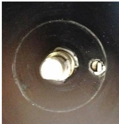
Figure 6 - Install Wiper Switch
