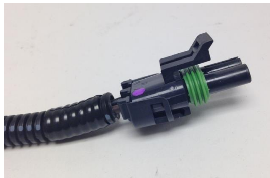
Figure 10 - Washer Pump Connection
