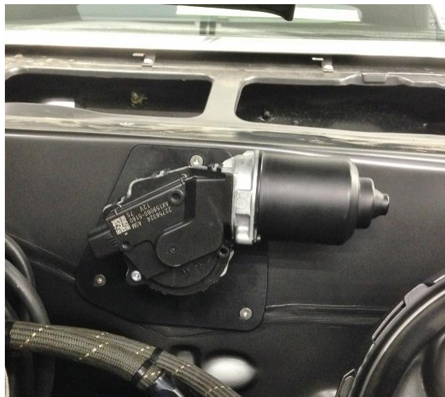
Figure 1 – Attach Wiper Motor to Firewall
