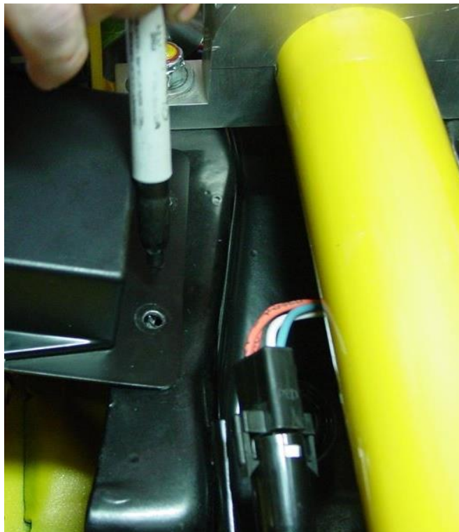
Figure 12 - Locate the Bolt Holes
