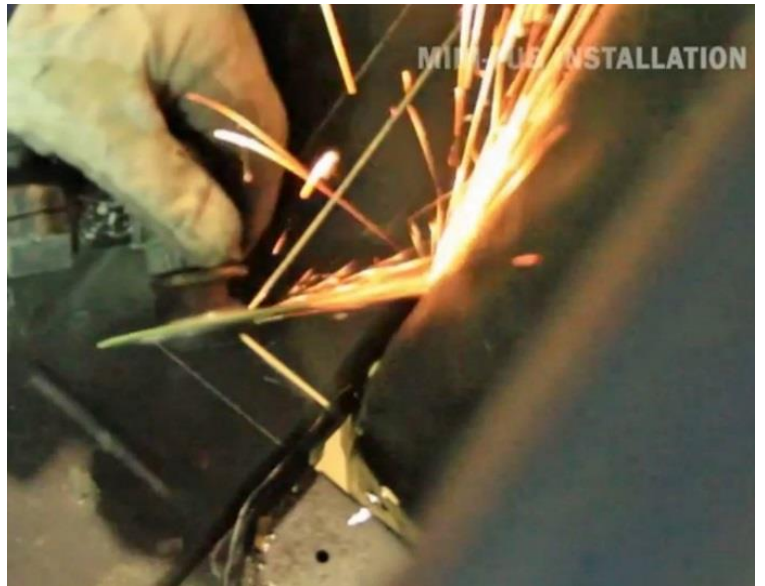
Figure 19 – Cutting the Inside Floor Pan
