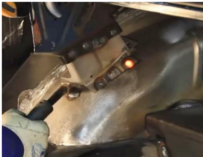
Figure 44 – Weld in Trunk Hinge Reinforcements.
