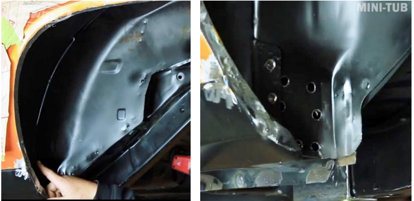
Figure 12 - Drill Wheel Tub Spot Welds
