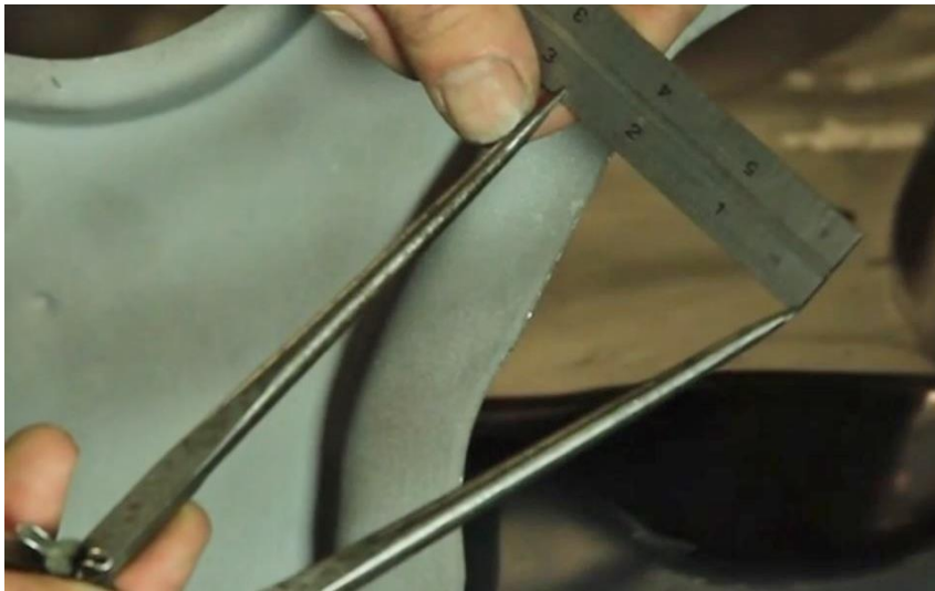
Figure 5 - Set Dividers and Transfer a 2-3/4" Scribe Line
