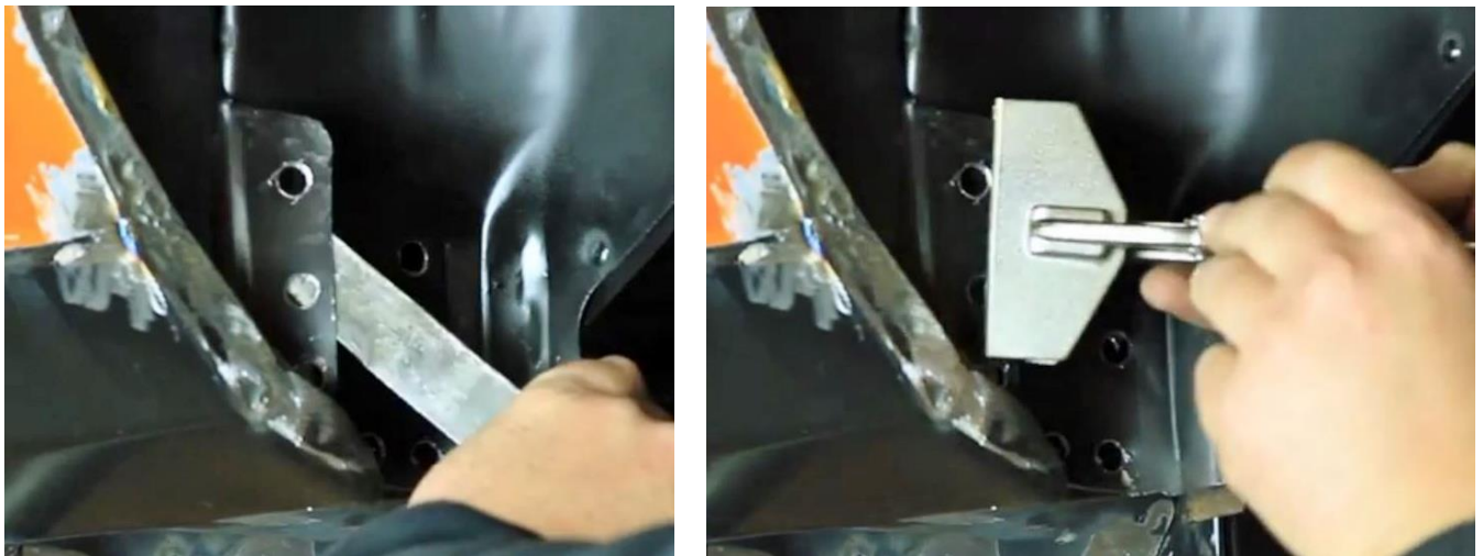
Figure 13 - Break the Seam Between the Outer and Inner Wheel Tub
