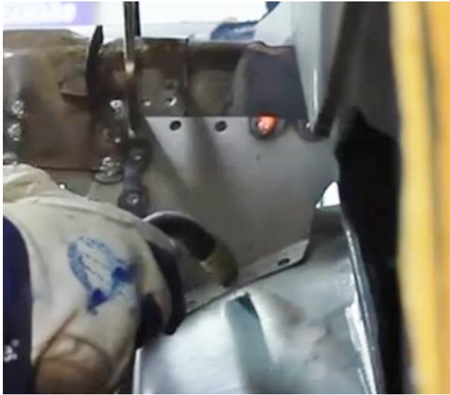
Figure 47 - Weld in Rear Seat Bracket Closeout
