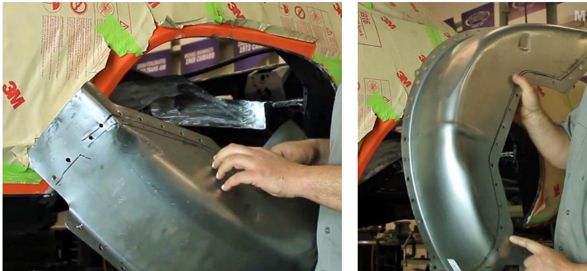
Figure 38 – Locate Plug Weld Holes
