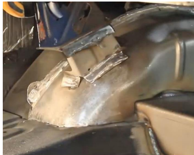
Figure 44 – Weld in Trunk Hinge Reinforcements.
