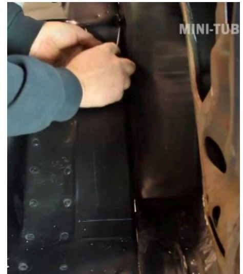
Figure 5 - Set Dividers and Transfer a 2-3/4" Scribe Line
