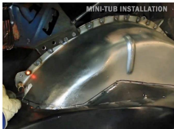
Figure 39 – Weld Detroit Speed Mini-Tub
