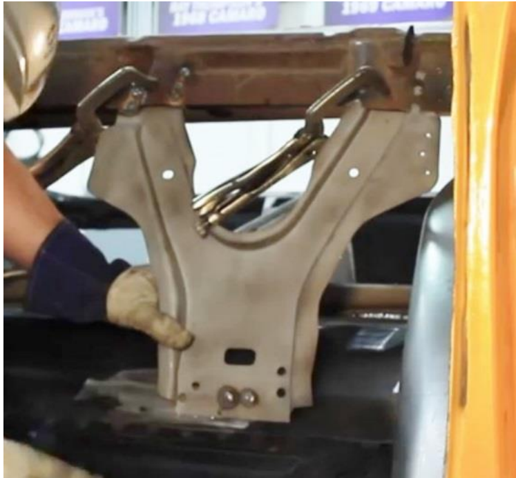
Figure 45 – Weld in Package Tray Reinforcements
