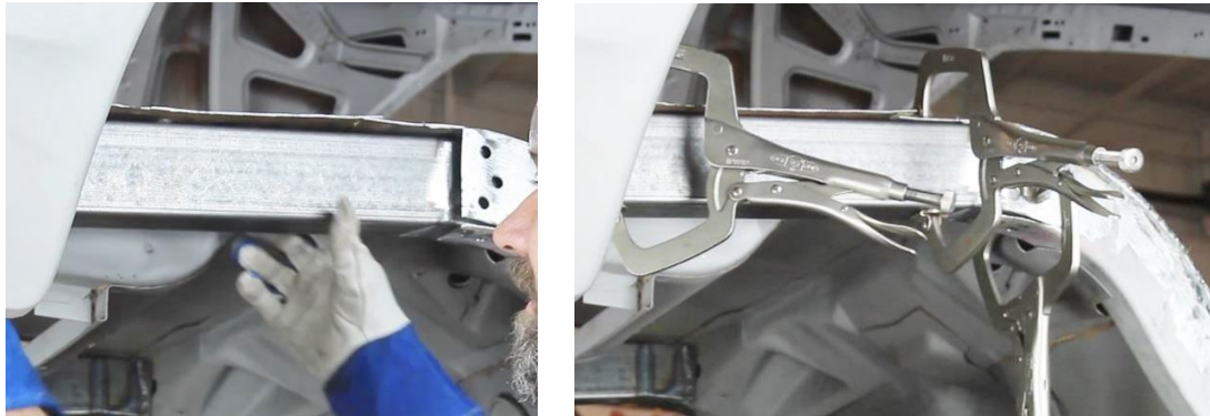
Figure 21 - Clamp Detroit Speed Frame Rail in Place
