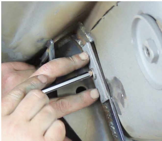
Figure 33 – Re-position the Seat Belt Anchor
