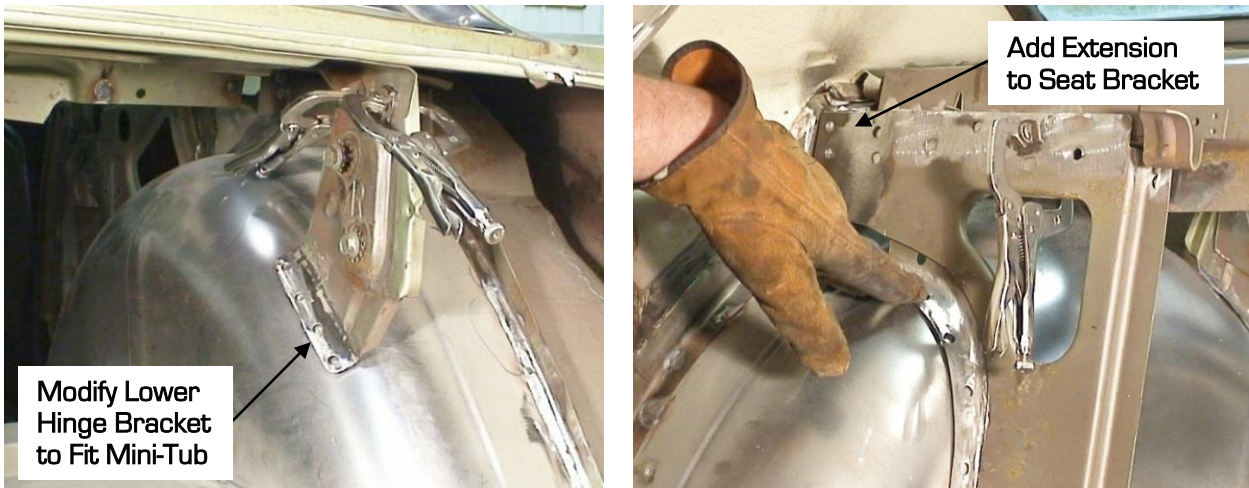
Figure 30 – Weld Rear Seat Support & Decklid Hinge to Mini-Tub (Coupe)
