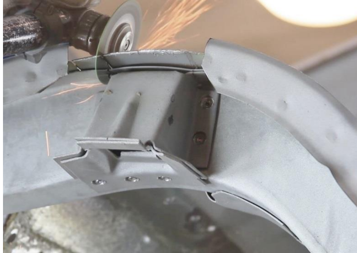
Figure 8 - Remove Bump Stop Bracket
