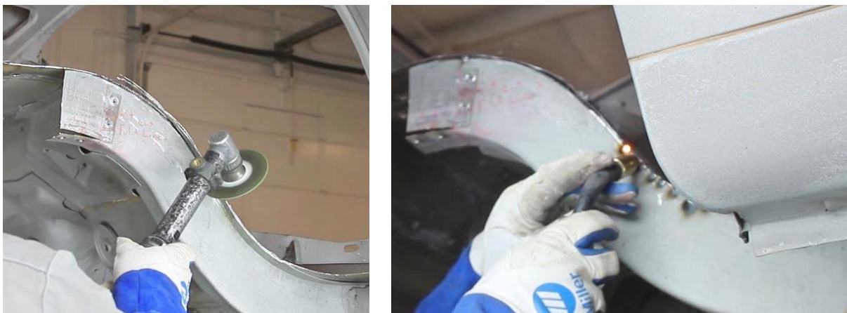
Figure 20 - Cut & Weld Sheet Metal Layers
