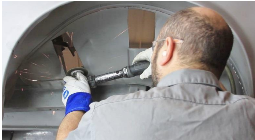
Figure 6 – Cut Out & Remove Inner Tub
