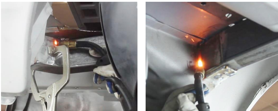
Figure 22 - Weld-In Detroit Speed Frame Rail Section
