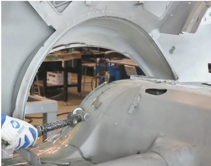
Figure 9 - Remove Floor Pan Section
