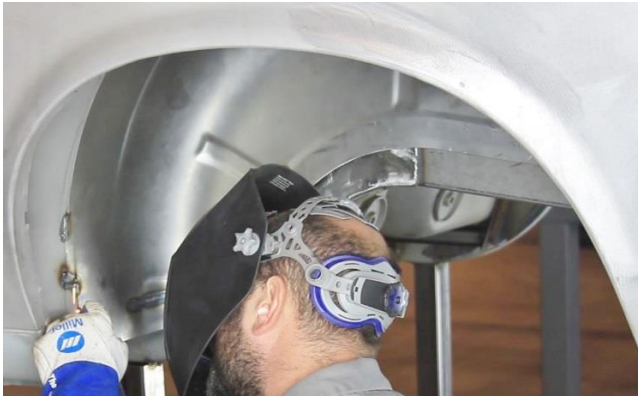
Figure 26 – Weld Mini-Tub to Stock Outer Tub
