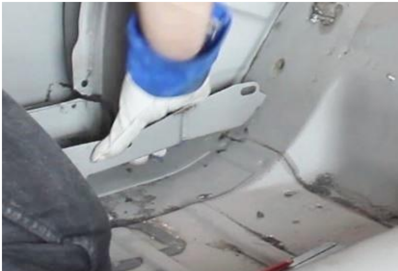
Figure 2 – Remove Interior Brackets
