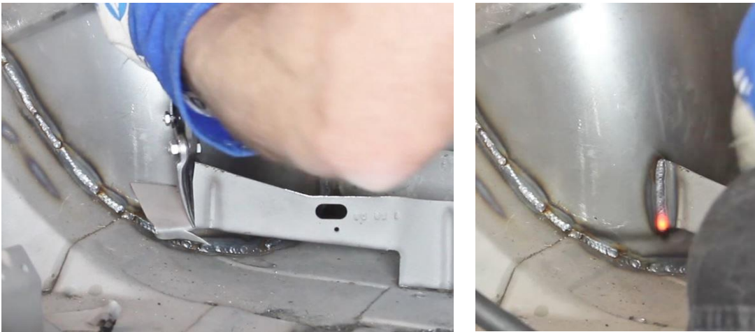
Figure 32 – Re-attach Rear Interior Panel Bracket
