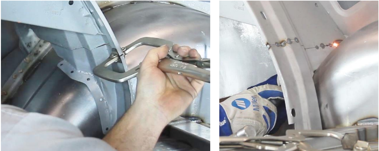
Figure 29 – Weld Rear Seat Support to Mini-Tub (Fastback)
