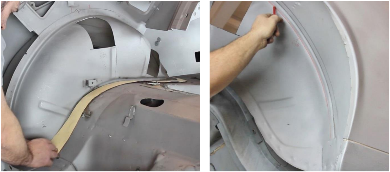
Figure 5 – Trace Floor Pan Cut Template
