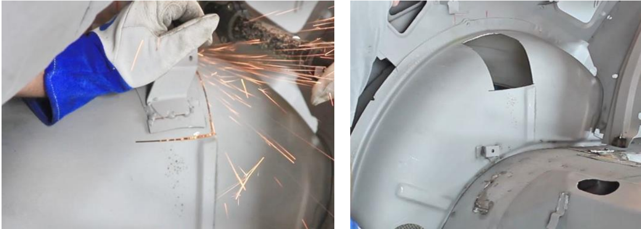
Figure 1 – Remove Lower & Upper Seat Brackets
