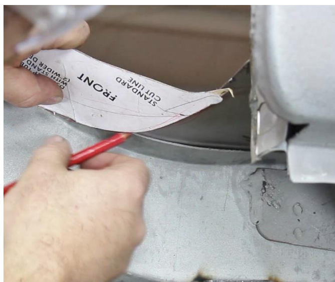
Figure 17 - Connect Frame Rail to Inner Tub Cut-Out
