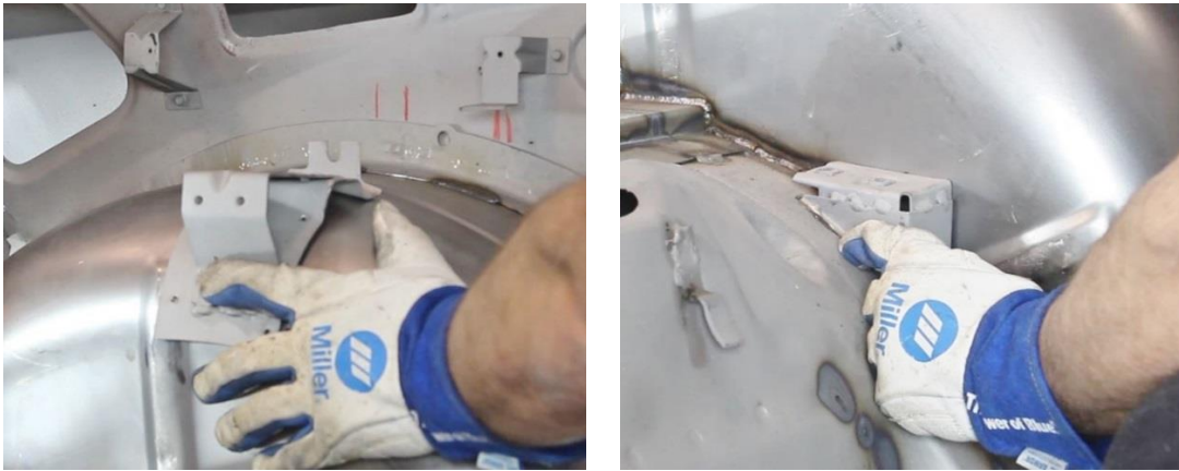
Figure 31 – Re-attach Upper & Lower Seat Brackets
