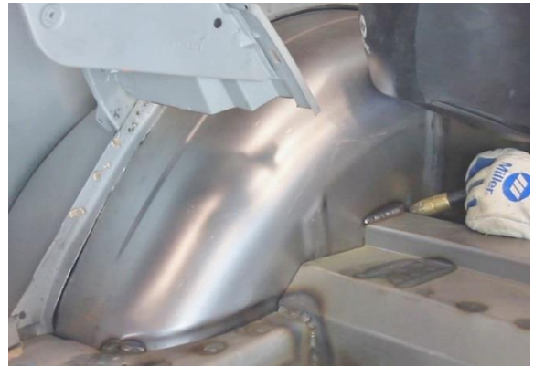
Figure 26 – Weld Mini-Tub to Stock Outer Tub
