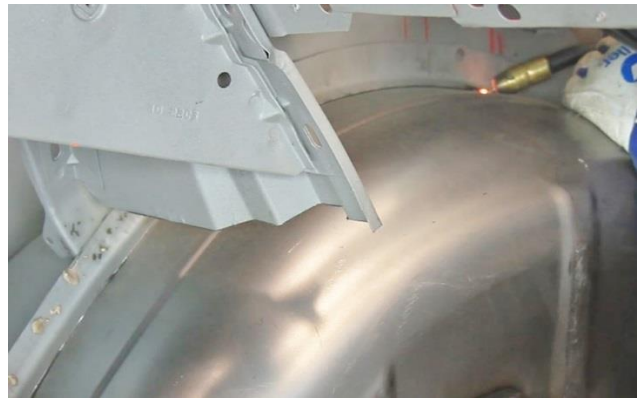
Figure 27 – Stitch Weld Mini-Tub to Frame Rail & Outer Tub Flange
